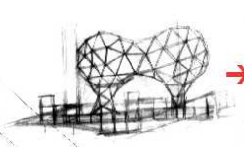
Structural Modules hold the floating concert hall and provide open air public space in different levels
