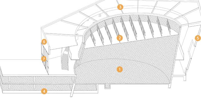
1. BEARING CONICAL TUBE MADE OF HIGH STRENGTH CONCILE.T
